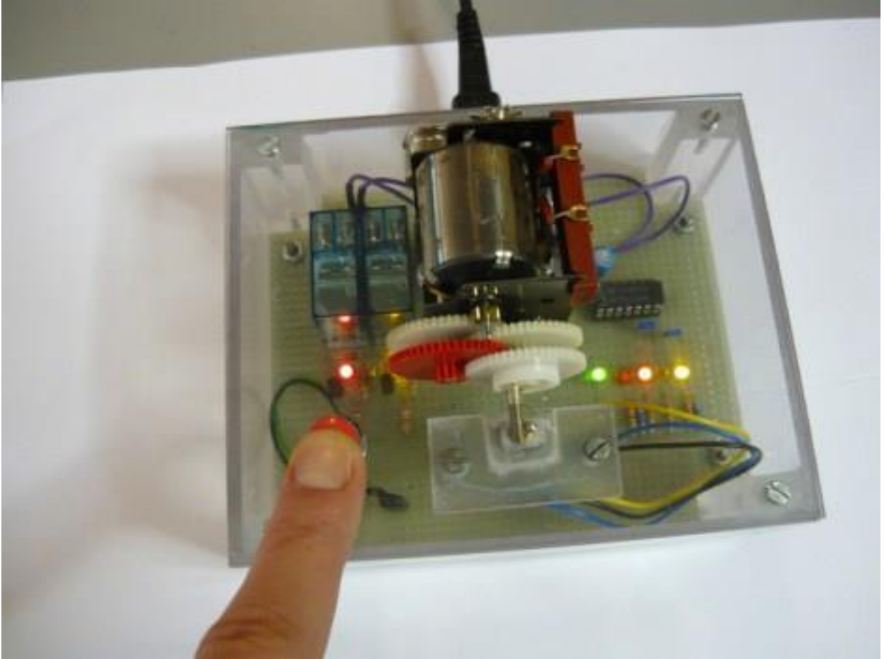
Figure 5.1.1. Example of the Bertho's pointless switch
